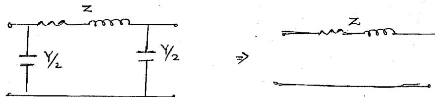
→ During short ckt fault the shunt element of x-mission line may carry negligible amount of current because of it's large impedance. so, in fault analysis always x-mission line will be represent as a short line model.
