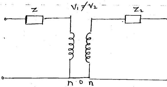
$Z_1, Z_2 \rightarrow$  leakage impedance of T/F winding.
